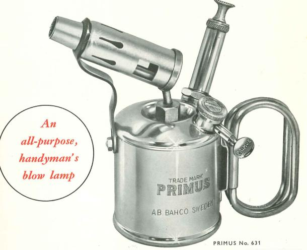
Primus Nos. 630 and 631 are popular because of their simple construction, reliability and easy maintenance. The efficient burner is suitable for most heating and soldering jobs, paint burning, etc.
